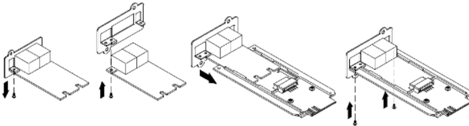
Step 1. Remove the screw holding the front panel to the card and remove the RMCARD205 front panel.
