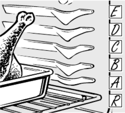
The oven has a special low rack (R) position just above the oven bottom. Use it when extra cooking space is needed, for example, when cooking a large turkey. The rack is not designed to slide out at this position.
