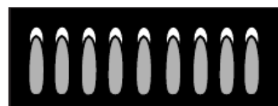
(B) Yellow tips on outer cones— Normal for LP gas
