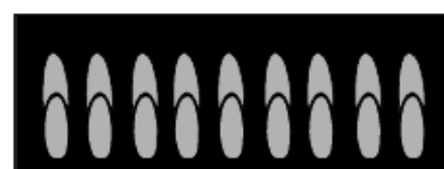
(C) Soft blue flames— Normal for natural gas
